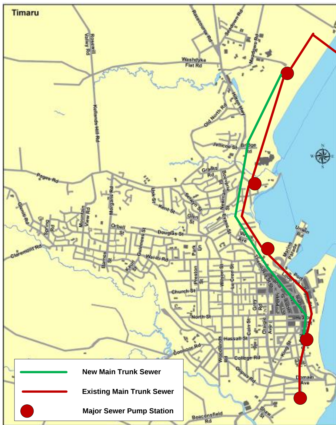
Figure 5.1: Overview Schematic of Timaru MTSR project
